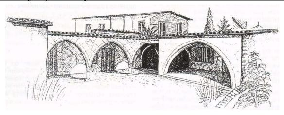
and the solarium absorbs and stores heat during the day and releases it during the night to the cooler exterior ambient air. The massive construction incurs damping and time lag of the high day temperatures.
